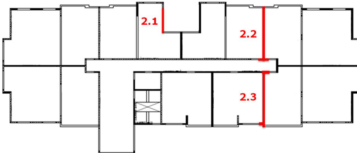
Figure A-4 Plaza del Rio Building B (Building No. 2) – typical floor plan with case study walls highlighted.
