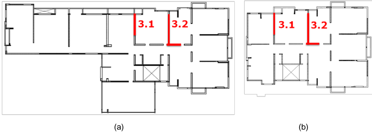
Figure A-6 Concepto Urbano (Building No. 3) – typical floor plans with case study walls highlighted: (a) ground through the tenth floor; and (b) eleventh floor through the roof.
